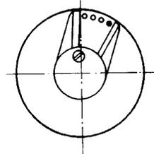
5. Next dividing operation: The shears are turned until the left arm touches the pin again; the next dividing operation follows as described in 4. above.
