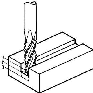
Most milling cutters are designed for peripheral work or slot cutting where the cutter is fed in from outside the workpiece edge. They are not designed for feeding into the workpiece from above to make a starting hole. When feeding into a workpiece from above you should always use a center cutting end mill. Feedrate for this operation should be no more than half that used for normal milling.
