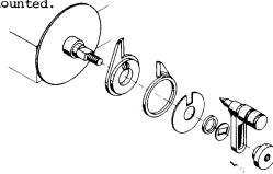
2. in the indexing table one sees that at the division 13, 3 full turns plus 3 holes on the 39 plate have to be added. Therefore, the shears are fixed so that they include 4 holes.
