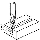
When depth of cut and feedrate are too great the milling cutter may bend, causing a danger of breakage. This is especially true with small diameter end mills and when slotting.
