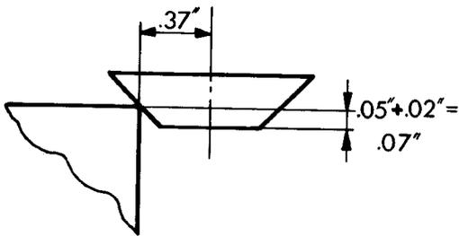
With an infeed of .07" the angle cutter touches the contour.
