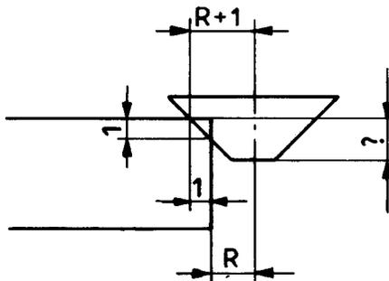
With a mill path using a 10 mm shank, dia. 12 mm, the radius of the angle cutter produces the chamfer 1x45°.
