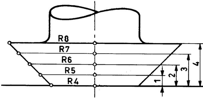
With a  $45^\circ$  angle cutter, the cutting radius changes by one mm if the cutter is fed in by 1 mm.
