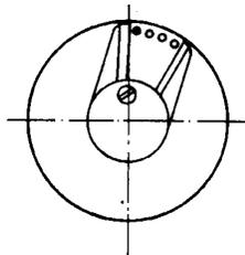
4. Execution of the dividing operation: 3 full turns plus the fractional turn of the 3 added holes are made; that means that the plunger is placed in the black hole. One dividing operation is completed.
