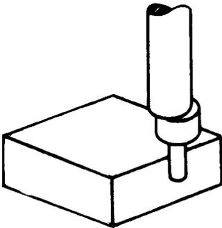
Now slowly jog the machine to move the edge finder near to the desired edge of the workpiece. When the rotating edge finder contacts the workpiece you will see the tip "jump" off-center about  $1/32$ ". At this point the centerline of the spindle is exactly .100" away from the edge of the workpiece.
