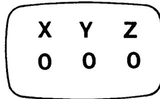
If you traverse in  $\pm X$ , the X lamp lights up. When you take your finger from the key, the traverse distance is shown in 1/1000" on the display. With a distance of 2.45" the display indicates 2450.
