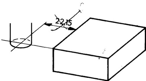
The center of the milling cutter is at a distance of 2.215" to the workpiece edge in X. The display indicates whatever value.
