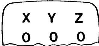
The display should indicate zero, when the milling cutter stands at a given point ( $X=0, Y=0, Z=0$ ).
