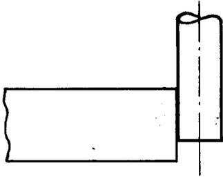
The contour is milled with a cutter of 10 mm dia.
