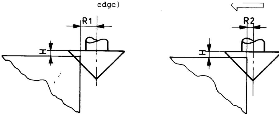
2. Chamfer size determined by different infeed and Z-direction. The cutter path remains unchanged.
