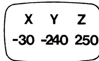
If you press the Z key, the light jumps to the Z lamp. After you lift your finger from the key, the traverse distance appears (with 1.000" 1000 will appear).
