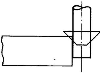
The contour is milled with a cutter of .500" dia.
