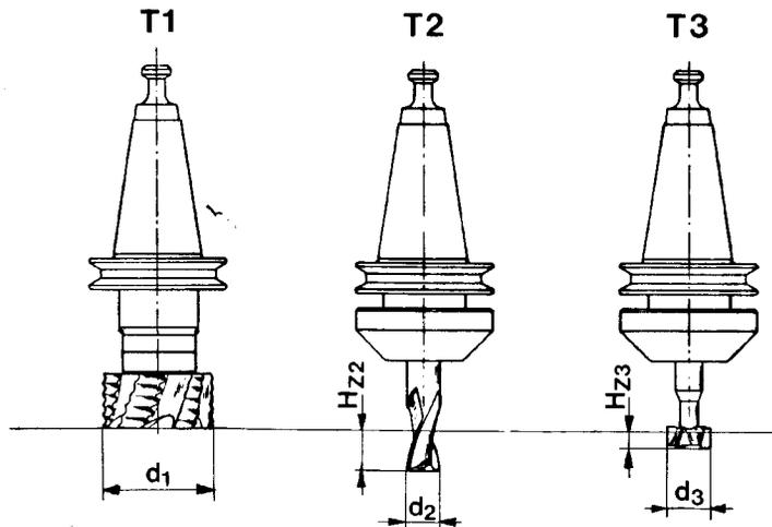
For the manufacture of a workpiece you often need different tools: drills, various milling cutters etc.
