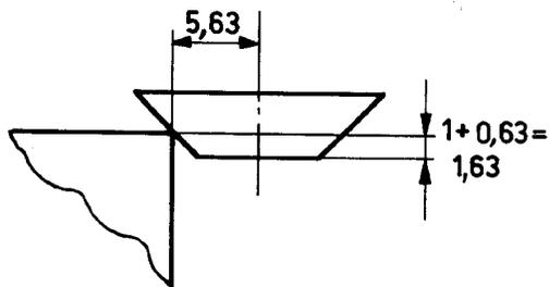
With an infeed of 1,63 mm the angle cutter touches the contour.
