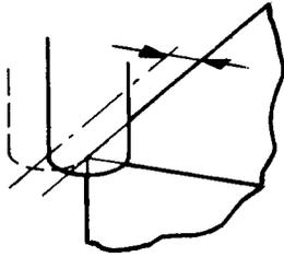
c) Touch milling cutter on front edge to scratch workpiece. Move milling cutter by value of milling cutter radius into X-direction. Set display to "zero".
