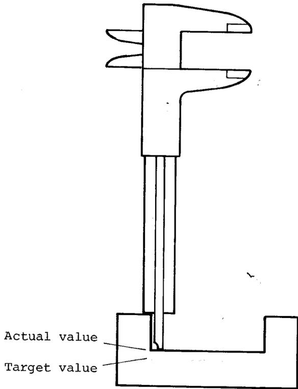
You have finished the manufacture of a workpiece and find out that the Z-measurement is not correct.
