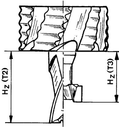
The differences in tool lengths have to be measured. The measurements can be taken using an external presetting device. In many cases the measuring system within the CNC-machine is taken use of.
