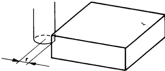
2. Scratch surface in X-direction. Put in value of milling cutter radius  $r$ .
