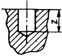
Blind holes are dimensioned down to the flat ground of the bore.
