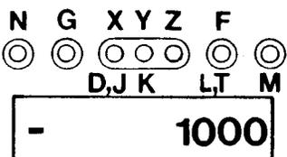
When moving at preset feedrate the display will change every 0.020" or 0.5 mm to update the position shown. In rapid traverse the display will not change until you lift your finger from the key.
